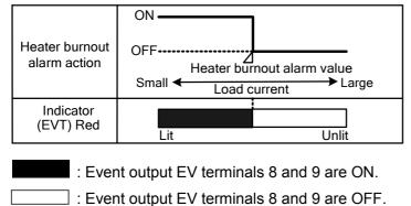
The Event output EVT indicator lights up when Event output EV terminals 8 and 9 are ON, and turns off when they are OFF.
