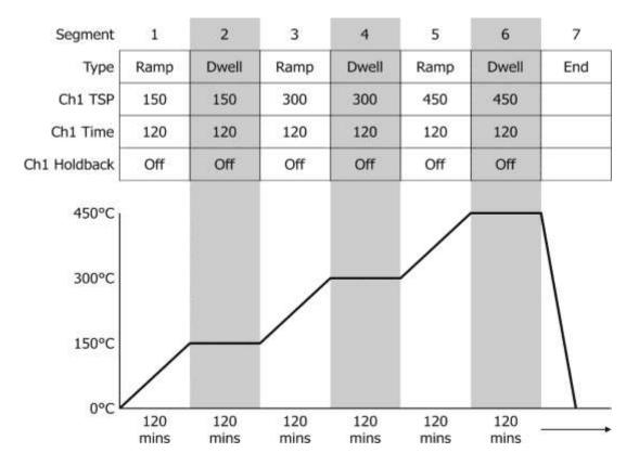
This PROGRAM has 7 segments and these segments are saved as TEST\_1 in the memory of the ADVANCED equipment.
