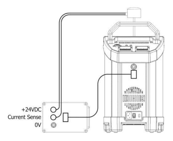
Connect the Transmitter to the equipment as shown in the above image.
